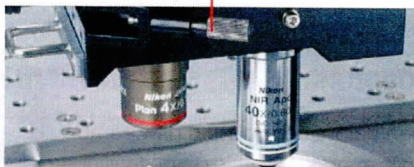
Parfocal distance correction knob
