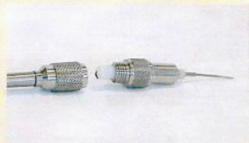
Insertion of Tungsten wire in electrode holder
